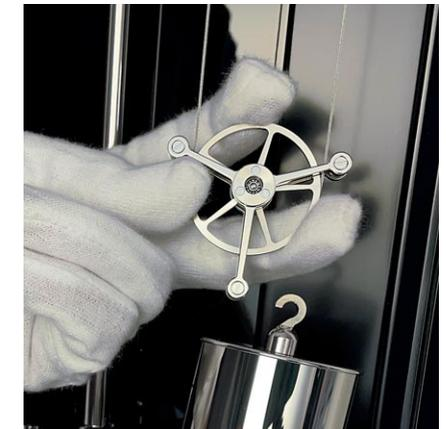
Wind the clock with the crank one turn counter clockwise. Deflect the pendulum until a "tick", caused by the drop of the escapement wheel tooth on the pallet, is audible. Watch the pendulum scale and note the angular minutes, indicated by the tip of the pendulum, exactly in the moment where the "tick" occurs. Now deflect the pendulum to the other side and again note the angular minutes when the "tick" is audible. It is ideal, when the angular minutes are equal on both sides.
