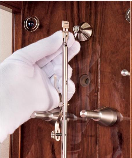
The pendulum tip should now point exactly to the "0 point" of the pendulum scale. The factory setting of the beat adjustment is made in this position.
