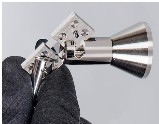
Push back the protection tube on the suspension spring block. Because of the lateral mounted air pressure compensation, the pendulum is pushed slightly from the centre position to the side. By turning the nuts at the sides of the pendulum scale you can adjust the pendulum scale in a position that the tip of the pendulum points exactly to »0«.
